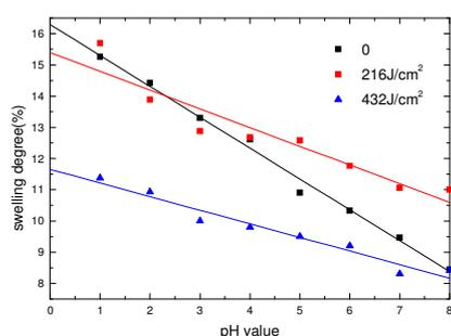
FIG. 3. Amount of swelling of poly(HEMA) versus the solution pH for different UV radiation exposures.
