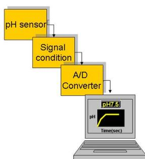
FIG. 2. Setup of the pH measurement system.
