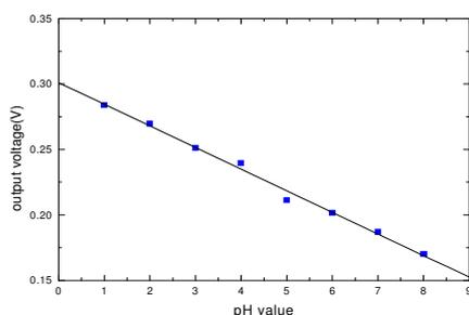
FIG. 4. Output voltage of measurement system versus the solution pH.
