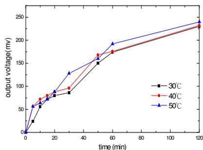
FIG. 5. Output voltage of measurement system versus time for different temperatures.
